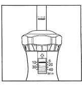
3. After adjusting torque setting, push down locking collar into "Lock" position.
