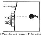
\* View the main scale with the angle perpendicular to the handgrip.
