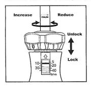
1. Pull out the locking collar for setting torque, turn Left to increase torque, turn right to reduce torque.
