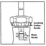
2. Torque setting is based on main scale plus locking collar scale. Adjust the locking collar scale, which is in increments of 1 ibf-in.
